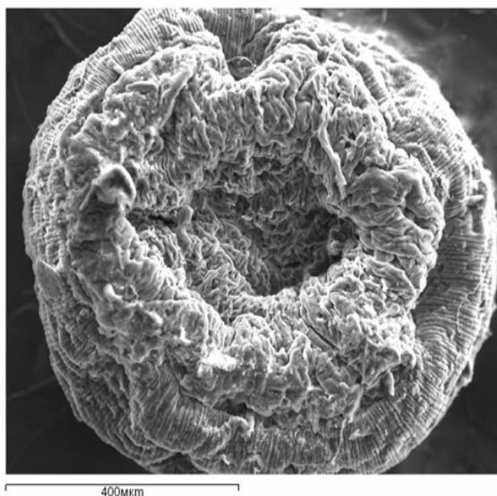
Figure 1 – SEM micrographs of the cytochrome-loaded alginate/chitosan microparticles
