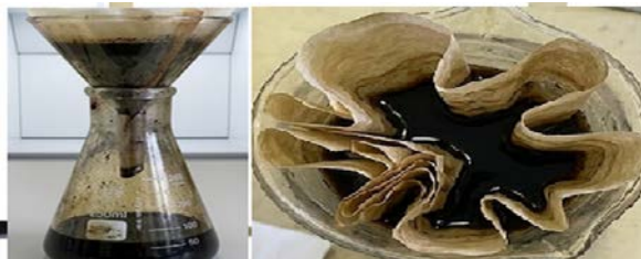
Figure 1 – Asphaltene filtration from Karazhanbas oil.
