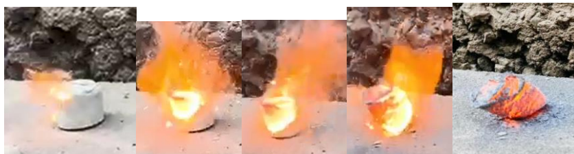
Figure 1 – Burning cinegram of a condensed mixture based on \text{TiO}_2 + \text{NiO} + \text{Mg}
