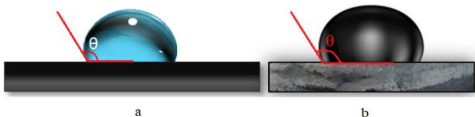
Figure 1 – Images of a drop on a solid surface: a – a drop of water on a bitumen film; b-a drop of bitumen on the surface of crushed stone.
