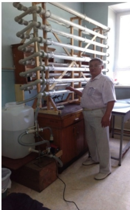
Figure 2 – Laboratory setup of the tubular photobioreactor
