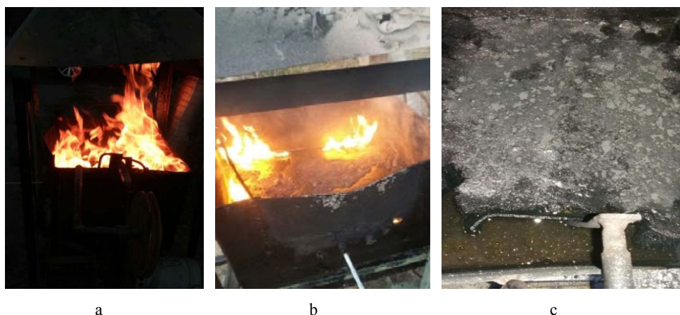
Figure 3 – Formation and use of innovative reagent formulations as a sorbent for the elimination of oil in a pilot plant: a) burning of oil on the water surface with different reagent compositions in the pilot plant; b) formation of thermogravite and reduction of combustion; c) adsorption of petroleum products
