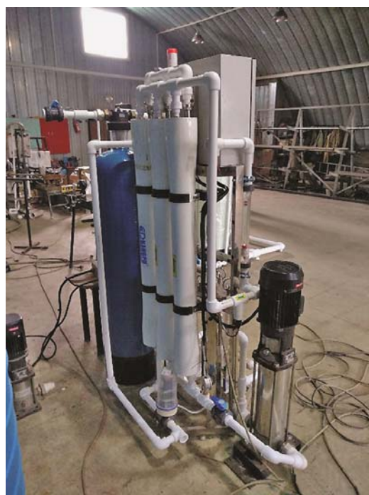
Figure 3 – General view of a pilot reverse osmosis plant with a capacity of 700 l/h
