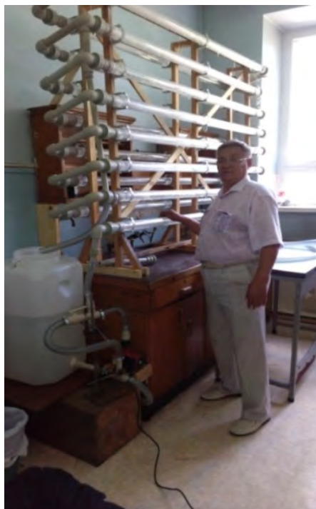
Figure 2 – Laboratory setup of the tubular photobioreactor
