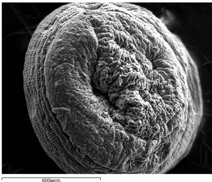
Figure 2 – SEM micrographs of the tilozine-loaded alginate microparticles
