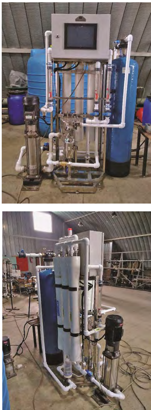
Figure 3 – General view of a pilot reverse osmosis plant with a capacity of 700 l/h
