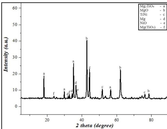
**Figure 5** – Results of the phase composition of the burning products of a condensed mixture based on  $TiO_2 + NiO + Mg$
