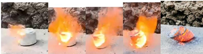
**Figure 1** – Burning cinegram of a condensed mixture based on  $TiO_2 + NiO + Mg$
