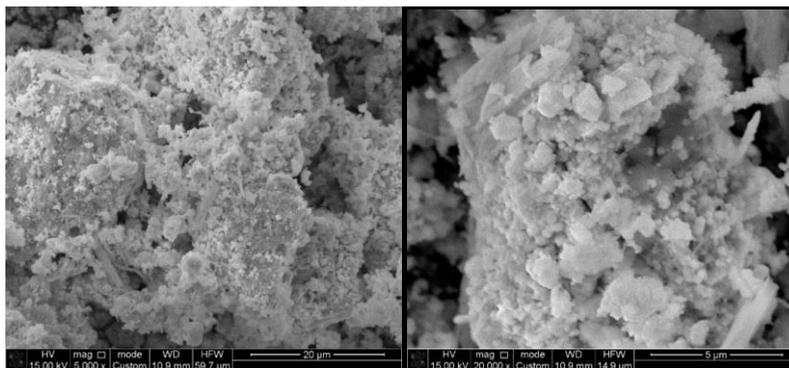
**Figure 6** – SEM analysis results of the  $TiO_2 + NiO + Mg$  system after the SHS process.
